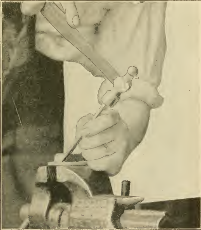
Fig. 74—Using a small chisel in removing superfluous metal from a small casting
